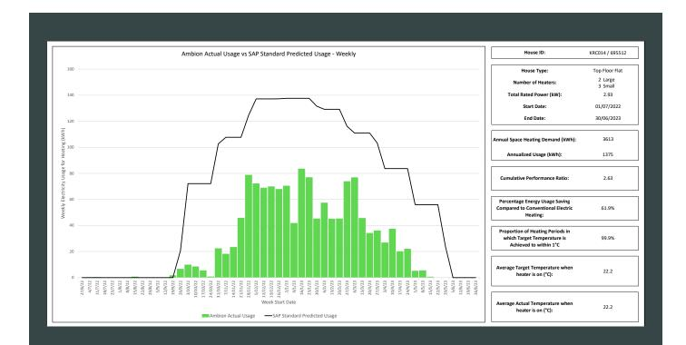
Each Ambion Low Carbon Heat Panel transmits hourly data to the Control Panel. Data is transmitted to the Ambion servers via the internet. This means that real operational data is routinely collected for Ambion systems, and can be used to produce reports.
